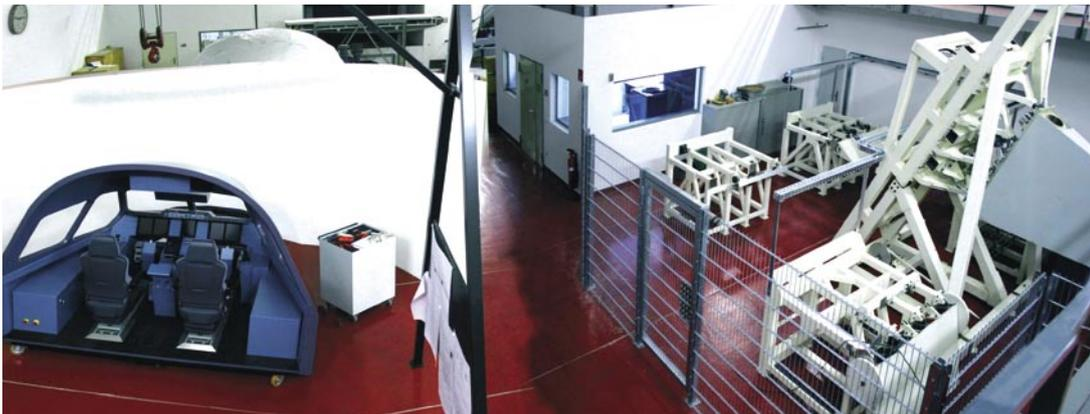
▲ *The iron bird at the German Aerospace Center (DLR) allows a wide range of flight situations to be simulated. The control surfaces are on the right, the cockpit at bottom left.*
