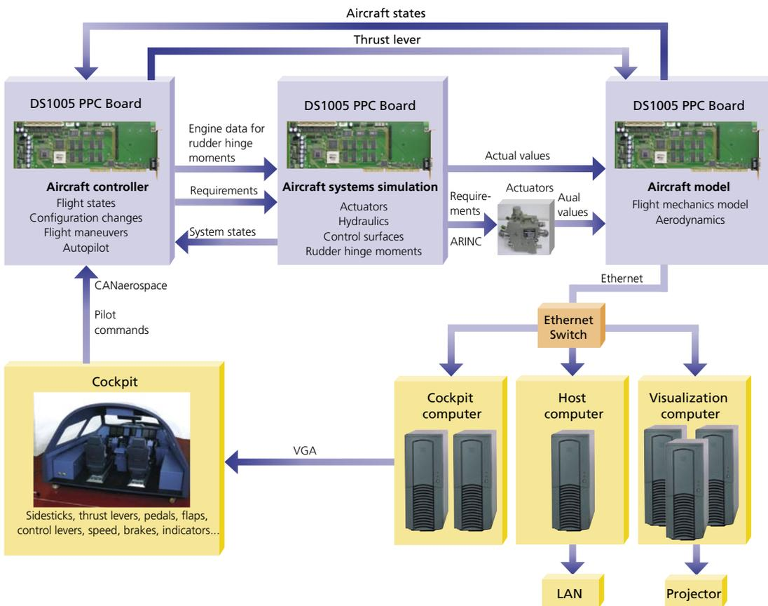
◀ *The multiprocessor environment consists of three DS1005 PPC Boards and performs calculations for the real-time simulation of flight maneuvers, hydraulic system, horizontal stabilizers, autopilot functions, automatic landing, and so on.*
